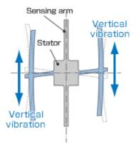
When the gyro is rotated, the Coriolis force acts on the drive arms, producing vertical vibration.
