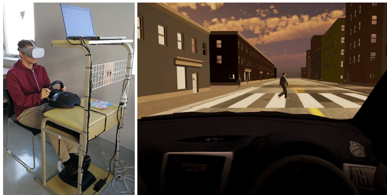
Fig. 1. Left: picture of the VR driving simulator including headset, steering wheel, pedals and the PC used to transfer data between them. Total cost of the whole equipment was below 500$. Right: screenshot of the scenario represented in VR; a pedestrian is seen crossing the road from inside the car.
