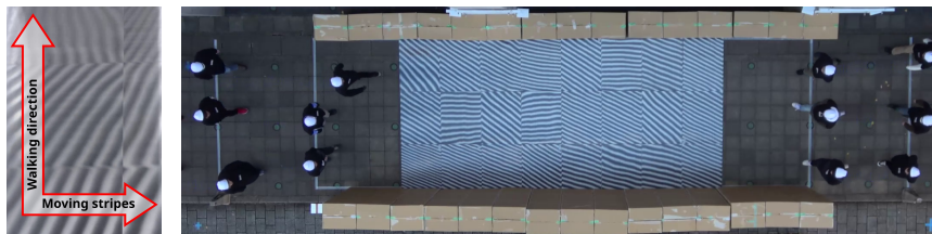
Fig. 3 Left: Working principle of the optical sheet, aiming to induce a turn to the right side. Right: Experimental setup used to check capabilities of the optical sheet in improving the smoothness in a bidirectional flow.
