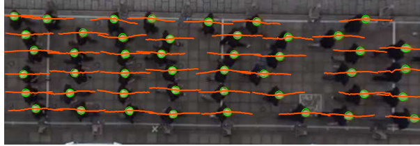
(b) Pedestrian recognition and tracking using PeTrack (Boltes et al. 2010; Boltes and Seyfried 2013) (trajectories are not complete).
